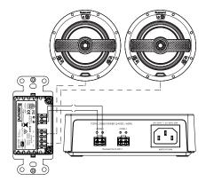
For a new installation, the location of the V-PS-2 power supply will be based on the wiring being done in the room and around the home at any other rooms. Each V-PS-2 can power up to 2 V-KP-1 wall-mounted amplifiers. Depending on the wiring that will be done at the home, it might be best to locate your power supplies in a central wiring location for the entire home, or in a central location for each floor or section of a home, or in a wiring closet near adjacent rooms, for example.
