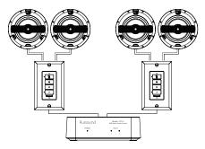
**The V-KP-1** is very easy to install and only requires two connections: power and loudspeakers.
