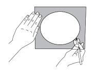
Use the enclosed installation template to illustrate the preference for the placement of the speaker as well as a guide when cutting the designated area.
