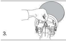
Connect the speaker cable to the speaker binding posts, which ensures that the polarity of the wiring is correct from the amplifier/source to the speaker
