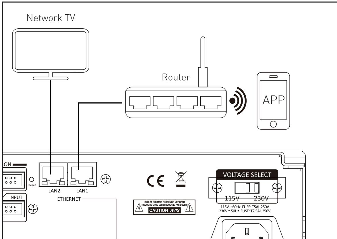
There are two RJ-45 jacks on the rear panel of this amplifier for the connection to Ethernet.
