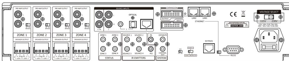
Once each unit is correctly addressed, use the provided ribbon cables to connect the OUTPUT of the original MASTER unit into the INPUT of Slave 1. To cascade the sources into a third unit, using the provided expansion ribbon cable, go out of the OUTPUT port from the device addressed as SLAVE 1 into the INPUT port of the device addressed as SLAVE 2.
