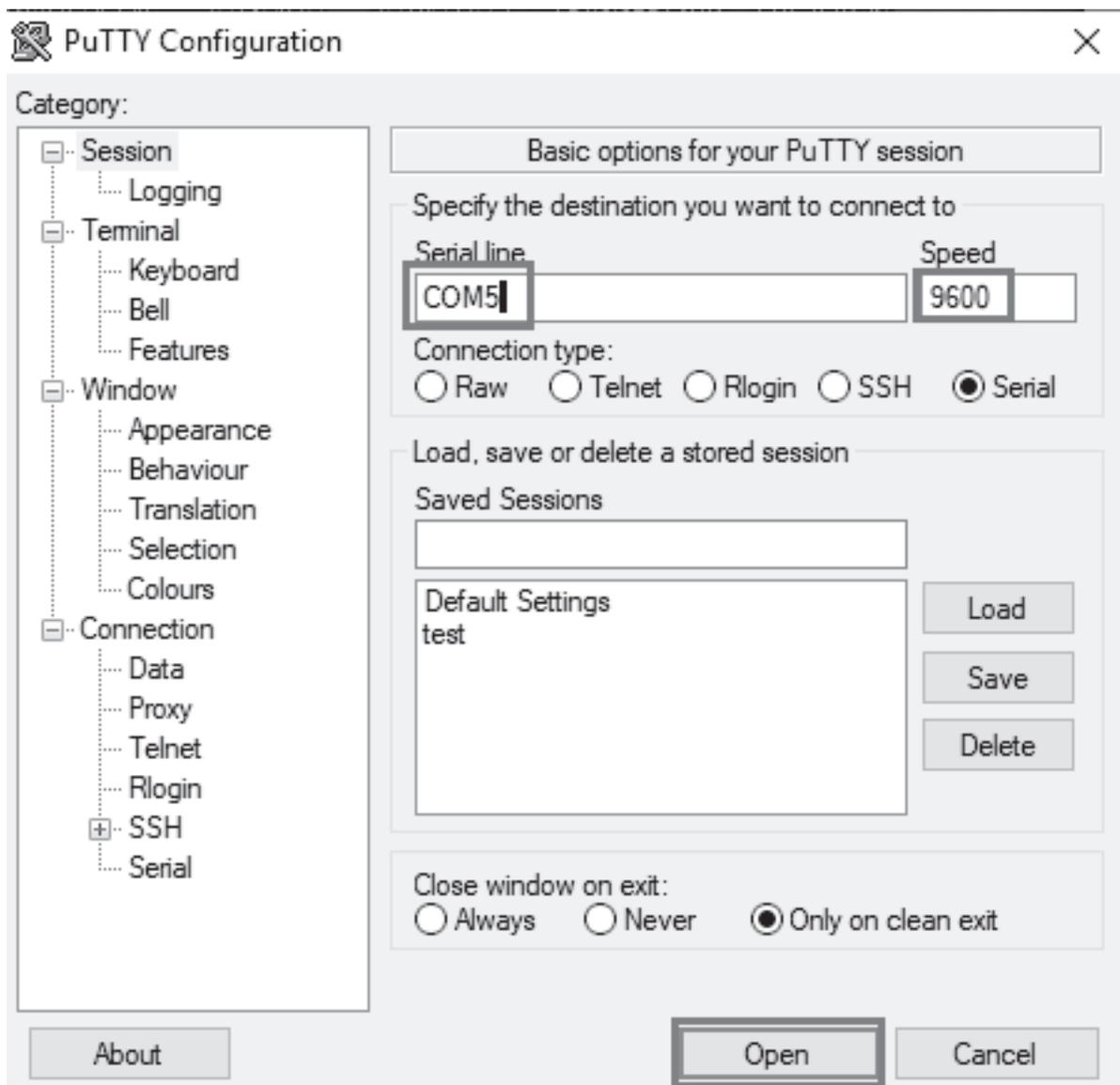
Click Serial, check the COM port and enter the Baud rate 9600.
