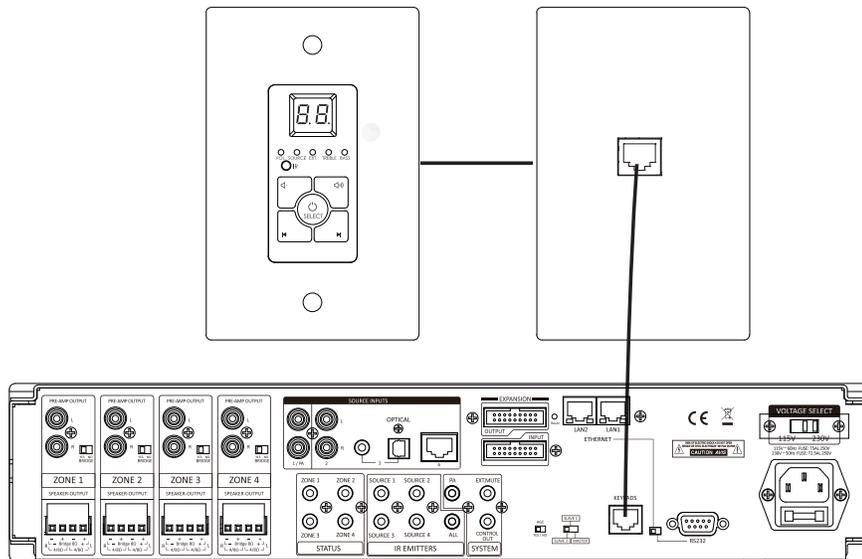
Without power being connected, connect a Cat5e/6 cable to the RJ45 port labeled KEYPADS on the back of the AMP. We recommend terminating the Cat5e/6 using the 568B standard.
