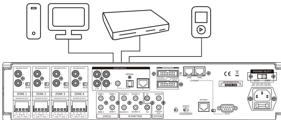
Some sources such as MP3 players and Cell Phones may require a 3.5mm Stereo to RCA Cables in order to connect to the AMP
