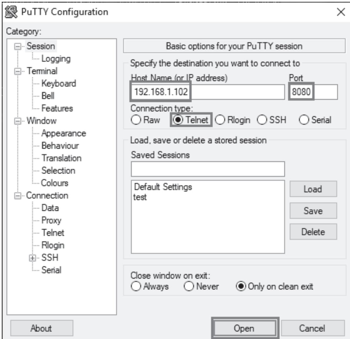
Click Telnet, enter the IP address of RX 800 and port: 8080.
