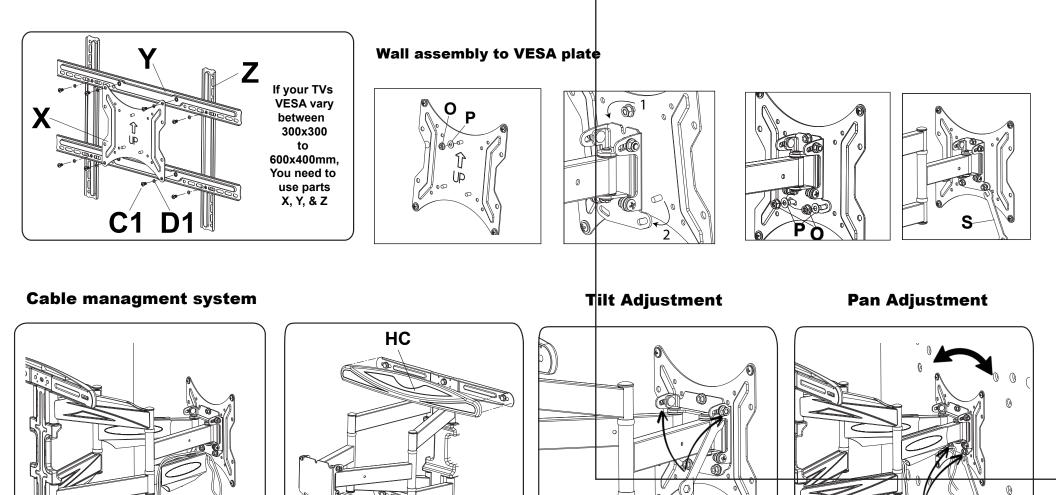
After tilt adjustment. Tight both ends of the nuts to secure it in place
